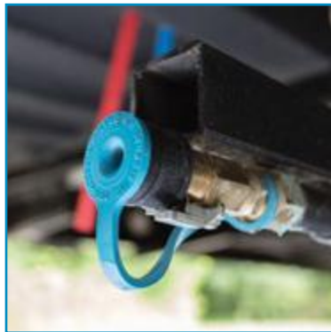
Exterior LP Connection
